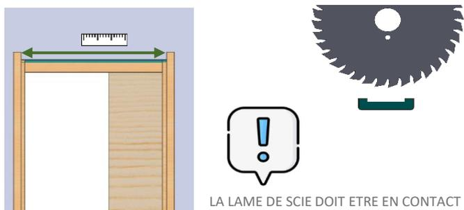
LA LAME DE SCIE DOIT ETRE EN CONTACT AVEC LA FACE OPPOSEE DE LA FINITION
